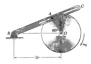
5. (10 Marks) (ILO b2.3) The hydraulic cylinder imparts motion to point B which causes link OA to rotate. For the instant shown where OA is vertical and AB is horizontal, the velocity  $v_B$  of pin B is 5 m/s and is increasing at the rate of 16 m/s<sup>2</sup>. For this position determine the angular velocity of OA.
