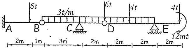
2- Calculate the reactions and draw the internal force diagram for the following beam
