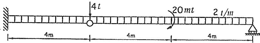
3- Calculate the reactions and draw the internal force diagram for the following structure
