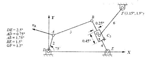
3. (18 Marks) (ILO c.13.2) If the velocities of points A and B are as given in the rigid body shown. Find the point C in that link at which the velocity is zero.
