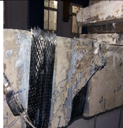
Fig. 2: RC beam post strengthening
