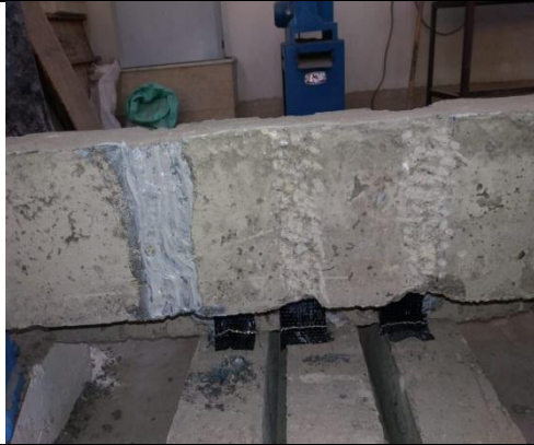
Fig. 1: RC beam prior strengthening
