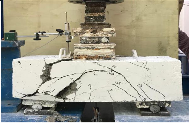
Fig. 3: RC beam cracks before reinforcement
