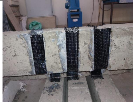
Fig. 2: RC beam post strengthening
