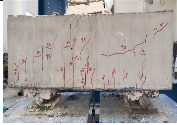
Fig. 4: RC beam cracks after reinforcement
