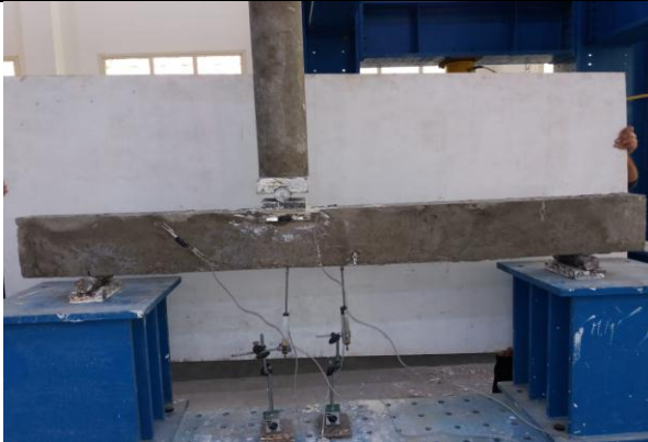
Fig. 1: RC beam prior strengthening
