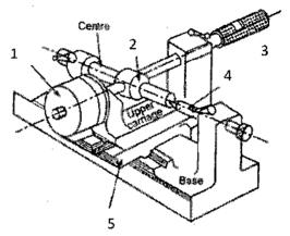
b) A floating carriage micrometer is an instrument that is used for accurate measurement of 'thread plug gauges'. List three gauge dimensions that could be measured using floating carriage micrometer.
