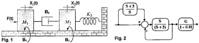
3. Find  $K_1$  and  $K_2$  for the system given by Fig. (2), such that  $M_p = 0.2$ ,  $t_p = 1$ , after that deduce the output time response for the given system.
