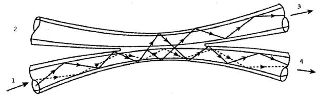
1- the excess loss is the ratio of power input to power output
