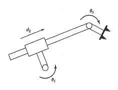
Find the 2 x 2 Jacobian that relates the two joint rates to the linear velocity of the origin of frame  $\{2\}$ . Give a value of the joint variables where the device is at a singularity. Ignoring gravity, what are the joint forces or torques required in order that the manipulator will apply static force vector  ${}^{0}F = 5\hat{X}_{0}$ .
