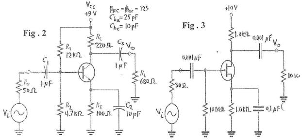
2. For the circuit of Fig. 3, Calculate the amplifier bandwidth if  $C_{iss}$ =10 pF,  $C_{rss}$ =3 pF,  $I_{DSS}$ =10 mA , $I_{GSS}$ =18 nA ,  $V_{DS}$ =-10 V,  $V_{GS(OFF)}$ =-8 V,  $V_{GS}$ =-3.36 V (12 mark)
