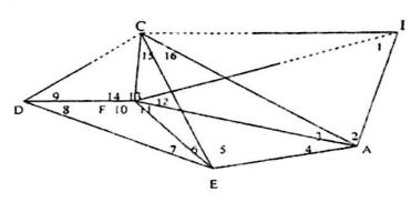
b) The field abstract for a triangulation scheme established for a small construction site is shown in figure. Using this data, calculate the adjusted angles.
