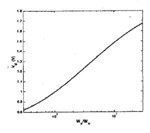
Explain and Analyze this curve to get observations about the Static CMOS inverter.
