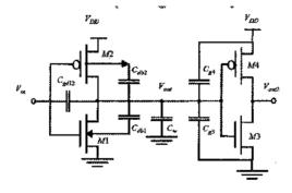
Analyse the parasitic capacitances using the Miller effect.
