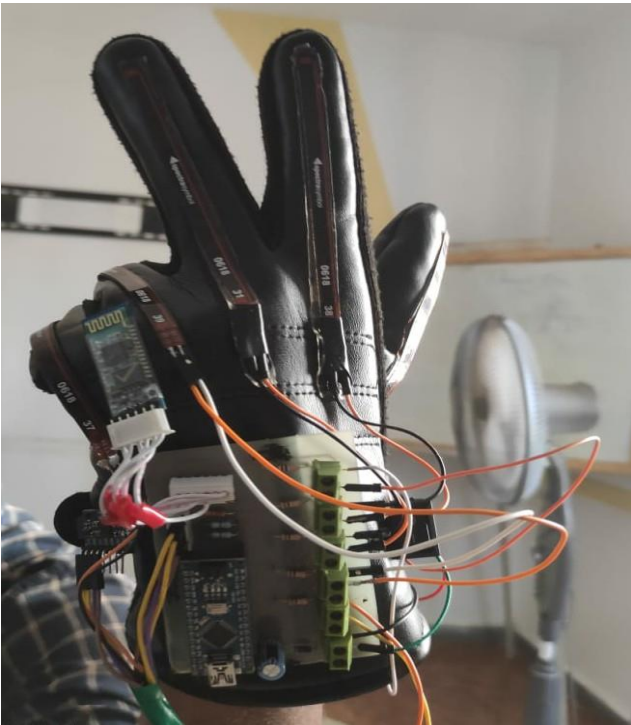
It is a glove that a deaf person uses to convert his hand signals into sound through
